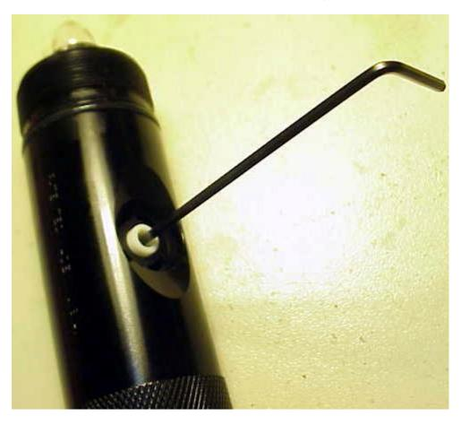
Unscrew it two or three turns and the switch drops right out the bottom:
