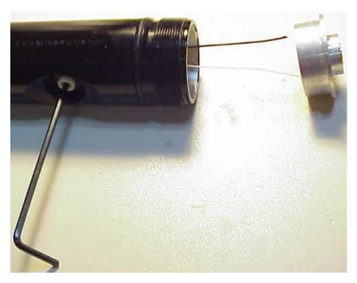
Apply thermal compound around the inside of the tube (where the anodizing was wirebrushed away), feed the two wires through the holes in the o-sink and press in:
