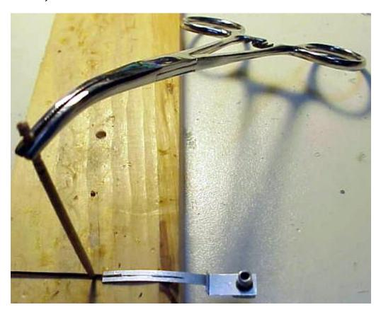
Notice I use a hemostat to clamp a toothpick, together the weight of which holds the wire down against the strip while soldering.
