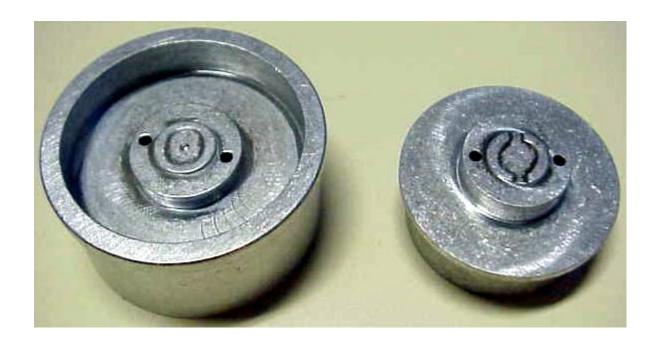
You can see that the machined central depression is of the exact shape as a Luxeon's bottom metal slug.
