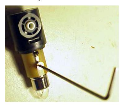
There will remain a long flat metal contact strip (with a threaded section at one end) for ground on the side of the switch body; it simply drops out the side. You'll need this later for the ground wire that goes to the Luxeon's negative lead.
