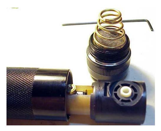
Use the same key to unscrew the focusing wheel and remove all the metal internals and discard (hint - push down slightly on the bulb to relieve pressure on the wheel while unscrewing):
